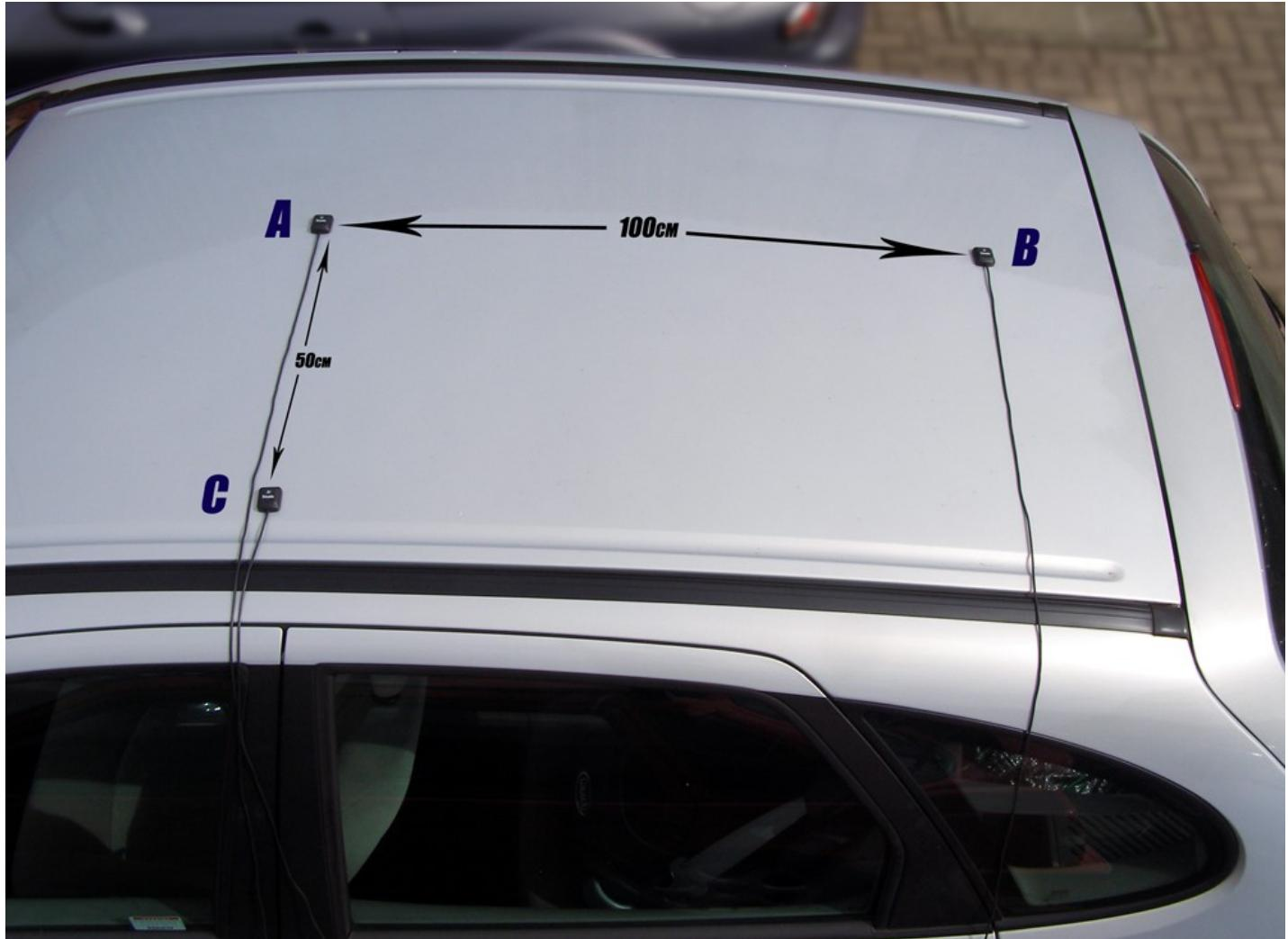
The picture above shows a typical 3-antenna placement for the measurement of Body Slip Angle, Pitch and Roll angle. Antenna A the primary antenna is placed in the centre of the roof. Antenna B is placed behind Antenna A, allowing True heading, Slip angle and Pitch Angle to be measured. Antenna C is placed to the side of Antenna A allowing the measurement of Roll angle.
