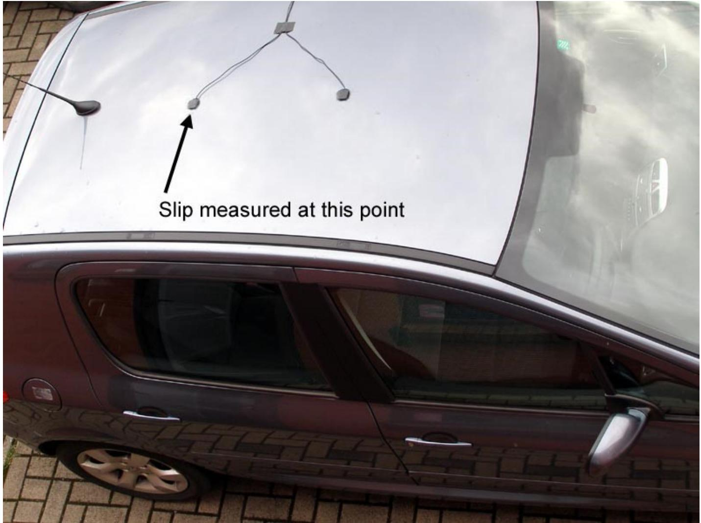
The picture above shows a typical antenna placement for the measurement of Body Slip Angle and Pitch angle.
