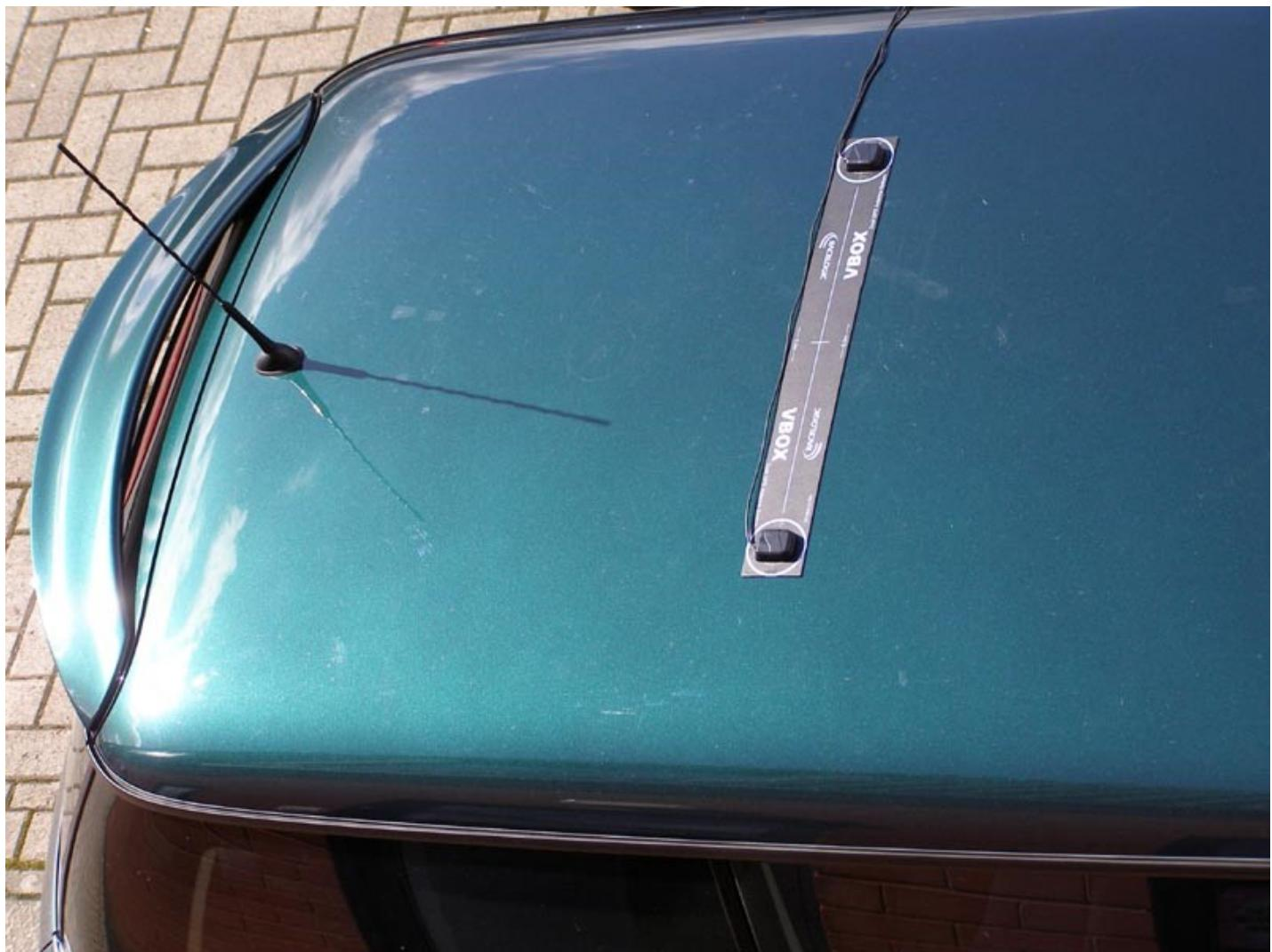
When measuring slip at a specific point on a vehicle (for example over a given wheel), the primary antenna must be placed over this point on the vehicle, whilst the secondary antenna should be placed towards the centre of the vehicle.
